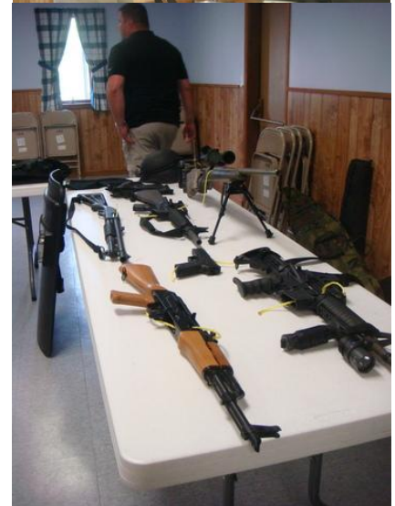
Yellow ties are used to show that the chambers are clear
